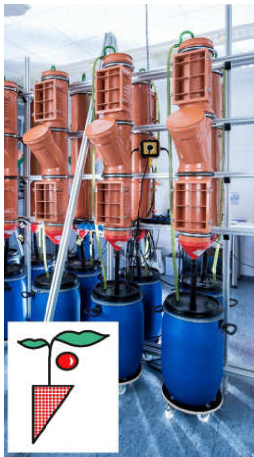
Fig. 3: The C.R.O.P. ® -biofilter for urine treatment. The blue barrel contains the urine which is processed by the microorganisms growing on the lava rock in the red tubes. A pump in the barrel circulates the urine through the tube bringing it in repeated contact with the microorganisms.
