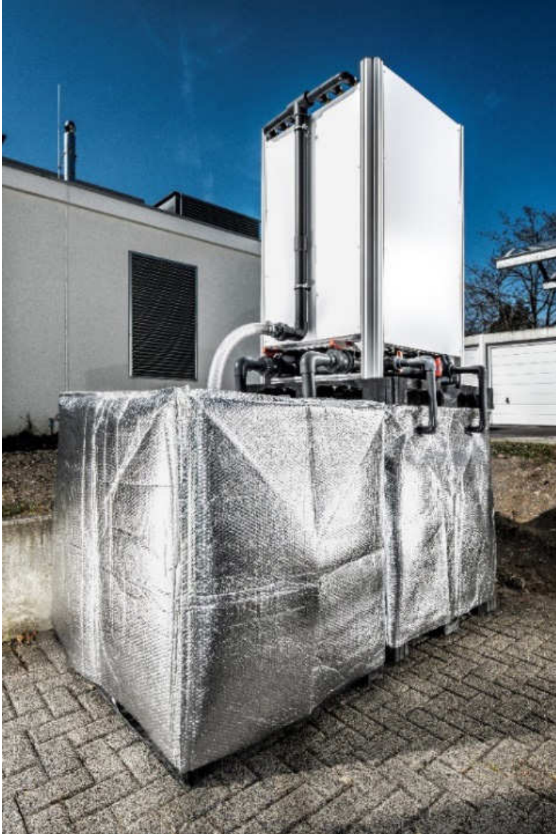
Fig. 2: First scale-up of a C.R.O. ® -biofilter in outdoor operation for the treatment of 100 l of cattle slurry per day.
